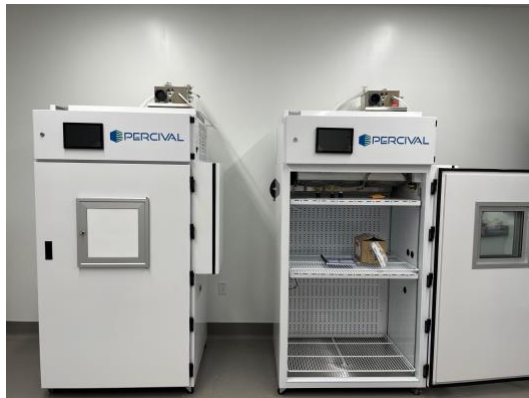
Figure 2. Two of the plant growth chambers where the class experiment will take place. Each chamber will be set up with its own CO 2 and temperature environment.
